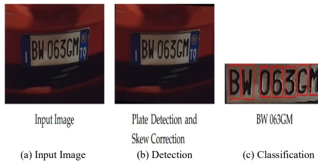
Fig. 6. The input image, detection, and classification of sampled license plate on vehicle
