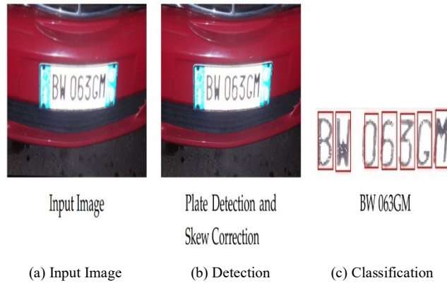
Fig. 7. The input image, detection, and classification of sampled license plate on vehicle
