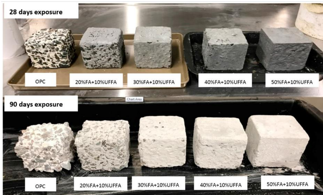
Fig. 3 Effect of acid attacks on the concrete samples with 3% H_2SO_4 solution [63].
